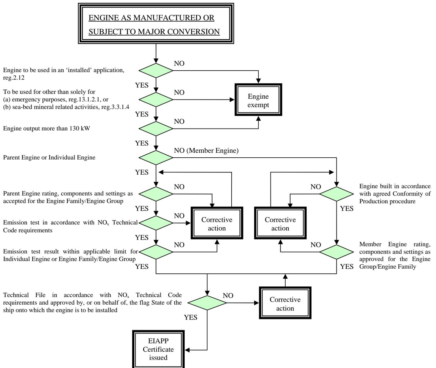
Figure 1 – Pre-certification survey at the manufacturer's facility
