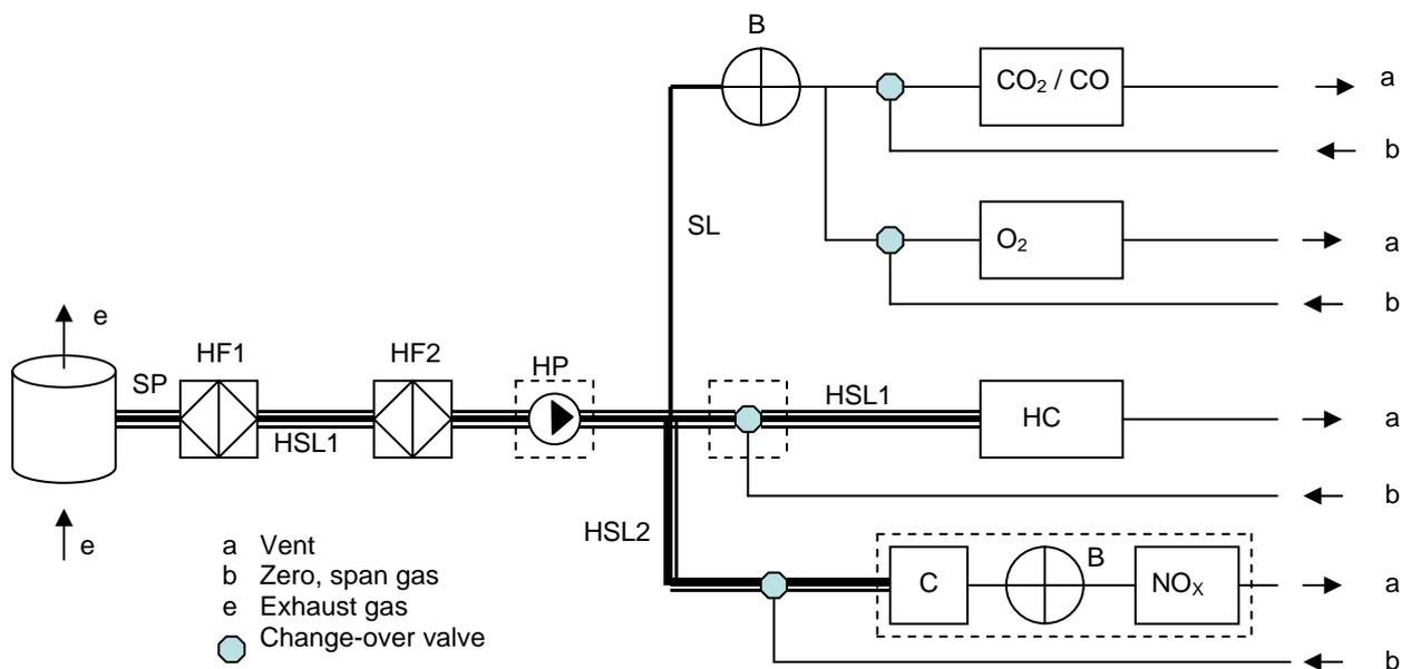
Figure 1 – Arrangement of exhaust gas analysis system
